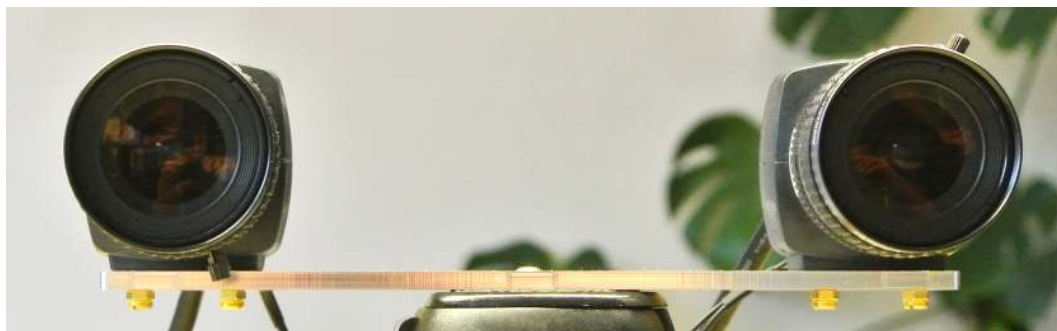
Figure 8: Example for valid stereo camera setup.
