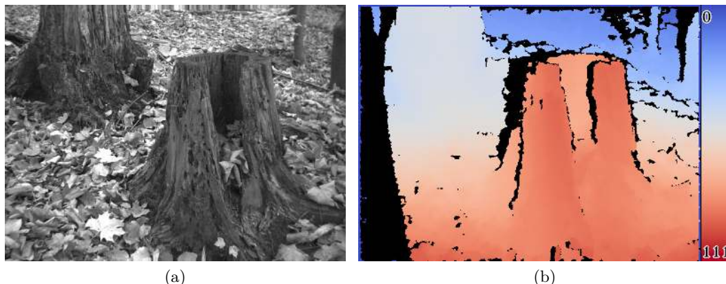
Figure 3: Example for (a) left camera image and corresponding disparity map.
