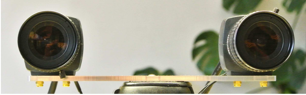
Figure 8: Example for valid stereo camera setup.
