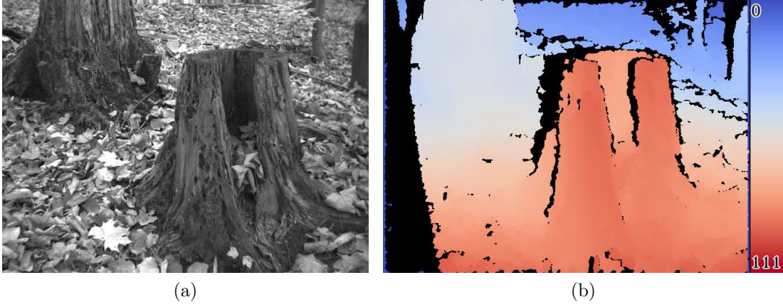
Figure 10: Example for (a) left camera image and corresponding disparity map.
