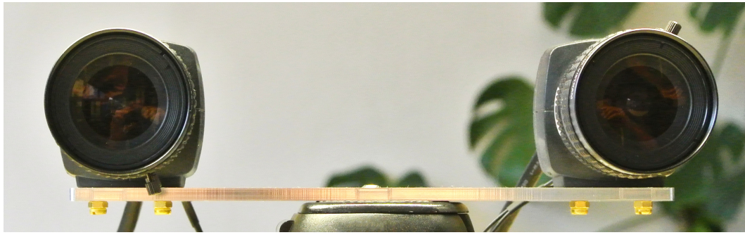
Figure 8: Example for valid stereo camera setup.
