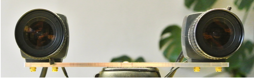
Figure 8: Example for valid stereo camera setup.
