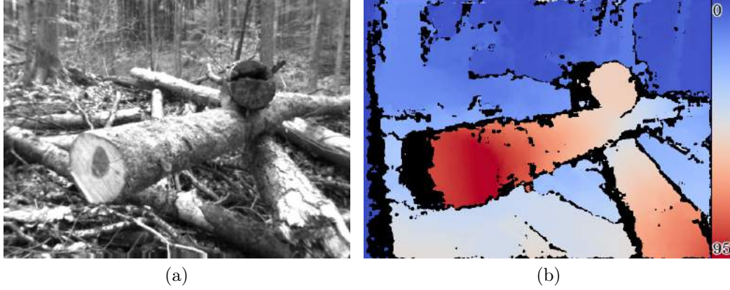
Figure 9: Example for (a) left camera image and corresponding disparity map.
