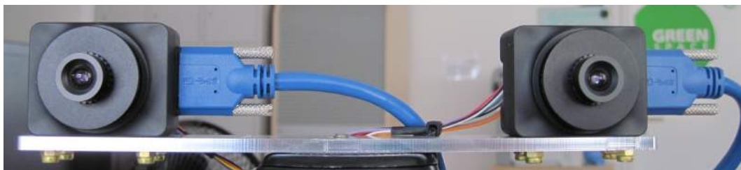
Figure 6: Example for standard epipolar geometry.
